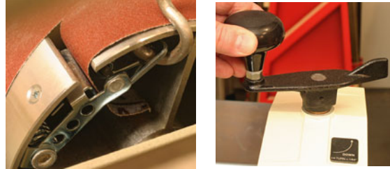
The optional TufTool™ (left) makes operating the take-up clip for the sanding strip easy. The large crank (right) changes the height of the sanding drum and makes tiny cut depth changes easy to make with precision.
