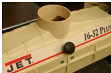
The 4"-diameter dust port molded into the upper shroud helps evacuate most of the dust.
