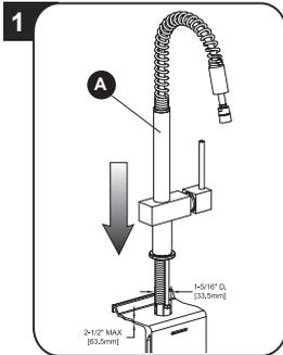
Before inserting the single lever group in the hole of the sink, make sure that the base gasket is properly positioned in its seat and that the flexible hoses are well tightened to the body of the tap. Place the single lever group in the hole of the sink, orienting the spout toward the sink tank.
