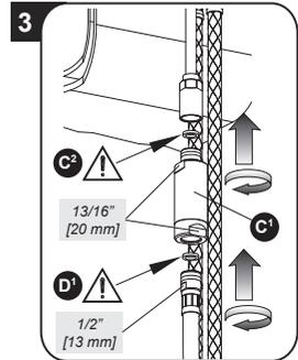
Install the check valve (C1) to the outlet hose with a rubber washer (C2). Secure with wrench. Attach the pull-down hose to the bottom of the check valve with a rubber washer (D1). Secure with wrench.
