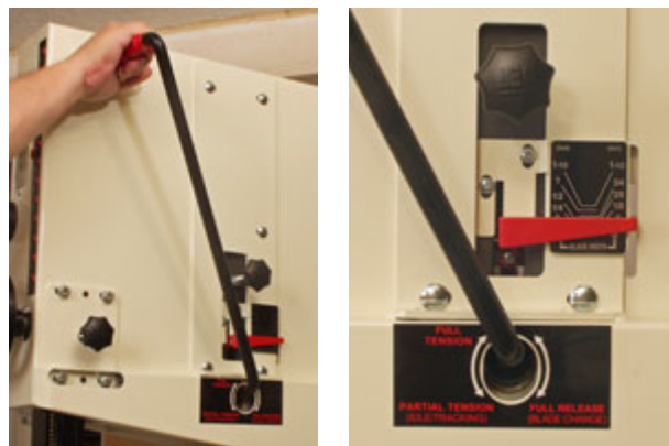
The long tension release arm (left) makes moving it between the detent positions very easy. Easy-to-read scales on the inside and outside of the upper cabinet make setting band tension quick and accurate.
