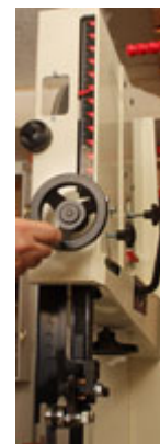
This rack and pinion drive raises and lowers the upper guide post.
