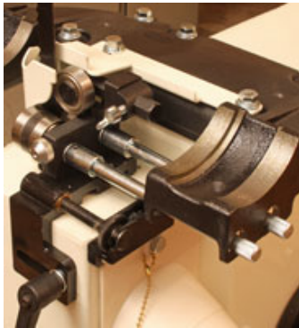
Fully adjustable and tool-free ball bearing guides are standard equipment at the bottom (left) and upper (right) guide positions. These fully sealed bearings provide great control and drag-free operation.
