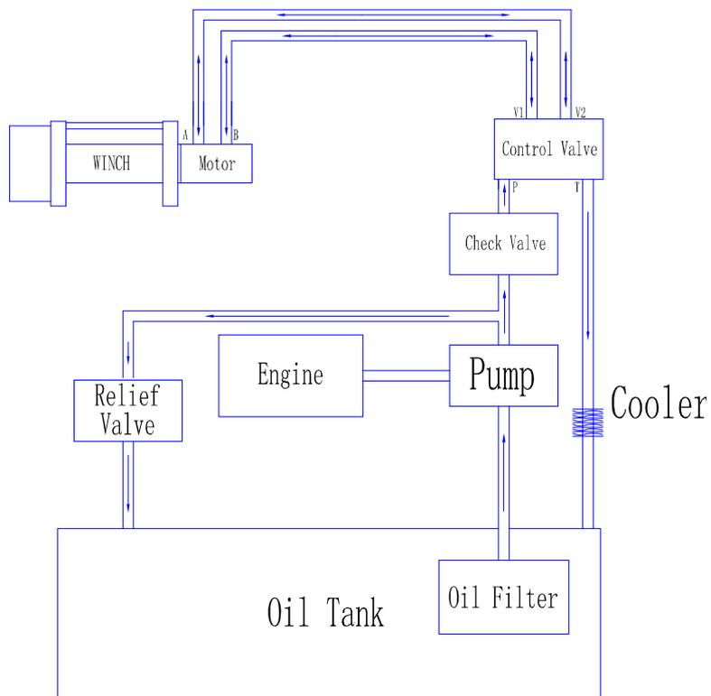
**Below is installation illustration of 10000NW:**
