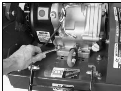
(E) Locate the four upper Engine Mounting Nuts on both ends of the motor and loosen.
