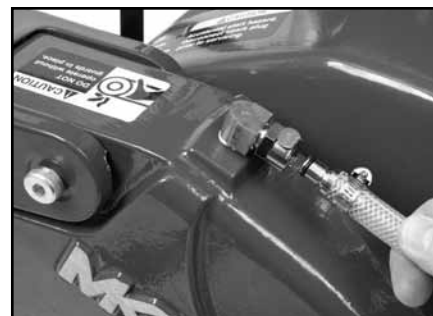
(I) Install the Cooling Transfer Hose from the Blade Guard.
