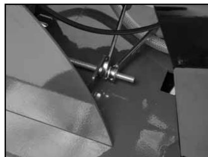
(H) Loosen the Engine Tension Arm adjusting nut. Push the Engine forward to loosen the belt.
