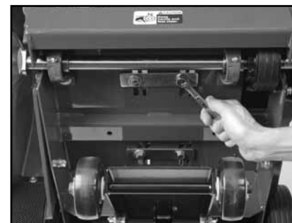
(F) Locate the four lower Engine Mounting Bolts on both ends of the motor and loosen.
