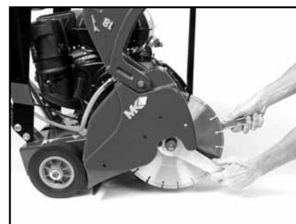
(H) Install Diamond Blade
