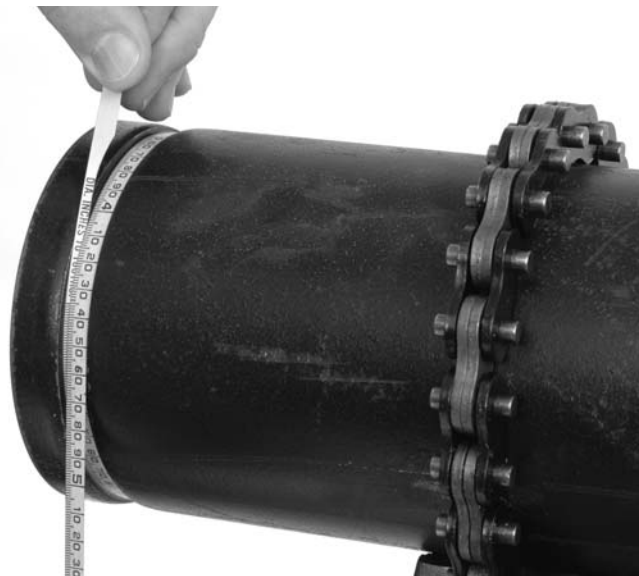
Figure 11 – Checking Groove Diameter With A Diameter Tape
