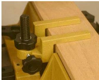
The material hold down is designed for ease of use and efficiency. Note the locking knob above the hold down that prevents loosening when the chisel is retracted.
