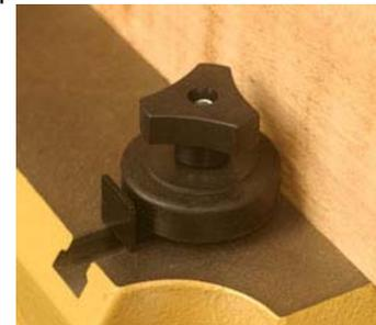
Roller-style material clamps keep the wood against the fence but allow repositioning for the next cut.
