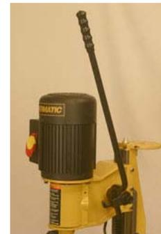
Other features include reversing the head for handling oversized projects off of the table (left) A 2" riser block for more over-table capacity (center) and an extra long, solid steel arm (right) That makes using the Powermatic 701 Benchtop Mortiser far less tiring.
