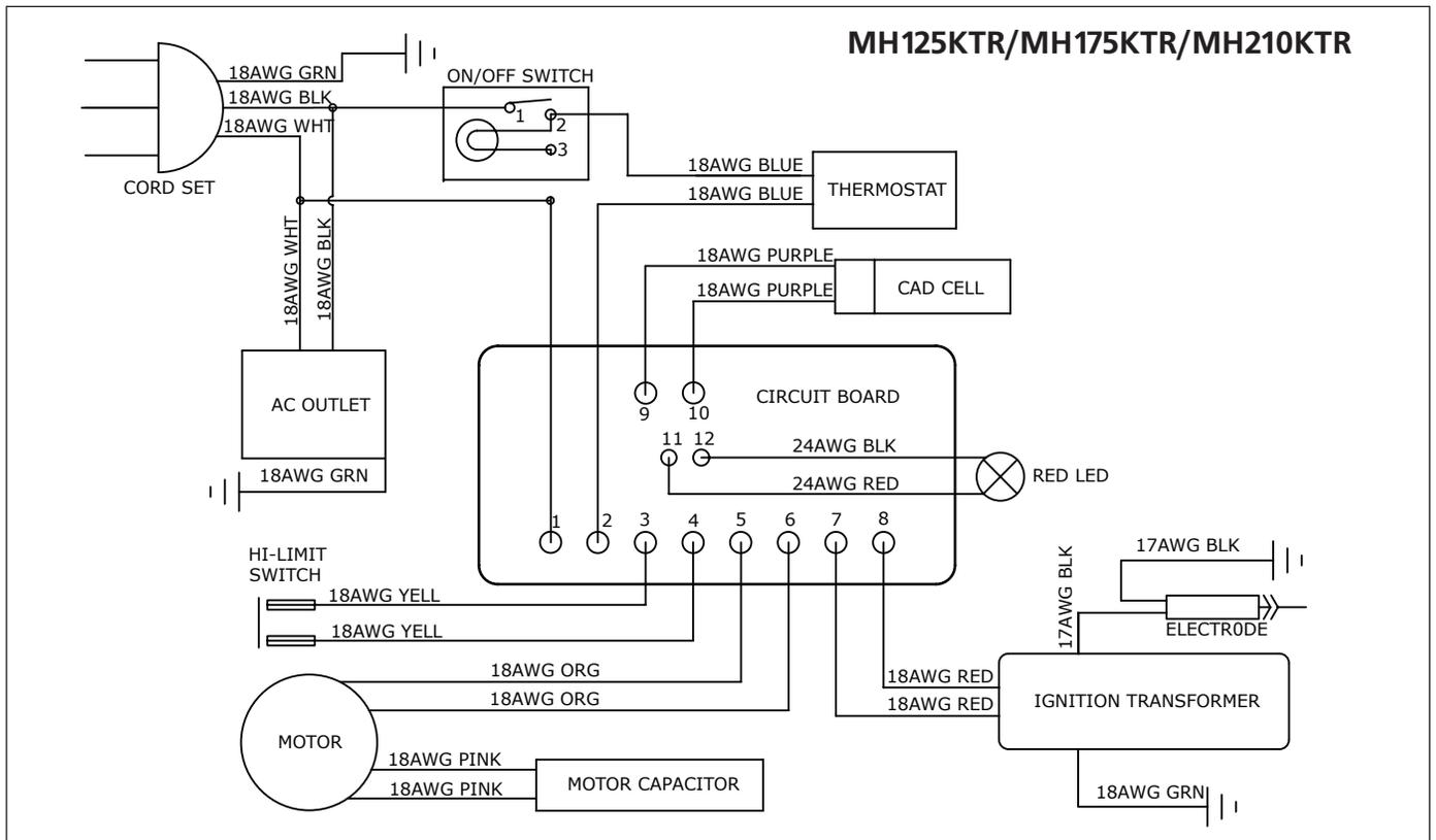
The parts lists and wiring diagram show the heater as it was constructed. Do not use a heater which is different from that shown. Heater performance is effected by air pressure setting. If there is any uncertainty about the air pressure setting,
