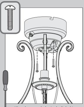
Align the screw holes in the light kit with the screw holes in the bottom of the lower switch housing and install the two light kit assembly screws, found in the hardware bag, to attach the light kit to the lower switch housing.
