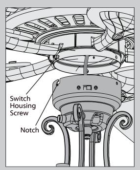
Align the notches in the sides of the lower switch housing with the screws on the upper switch housing. Lift the lower switch housing and twist clockwise to lock it into place.
