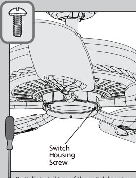
Partially install two of the switch housing screws, found in the ≡ hardware bag, into the screw holes in the side of the upper switch housing. It does not matter which two screw holes you choose.
