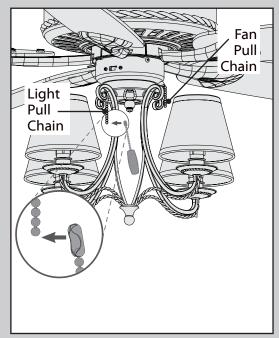
Connect the appropriate pull chain pendant to each of the short chains coming from the switch housing.
