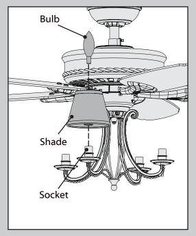
To install each shade, remove the plastic covering and place the shade over the socket so the ring in the center of the shade fits onto the socket, then install the bulb. When necessary, replace with bulbs of the same type and wattage.
