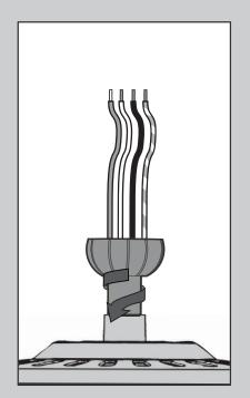
Hand tighten the downrod (at least 4-5 full turns) until it stops.
