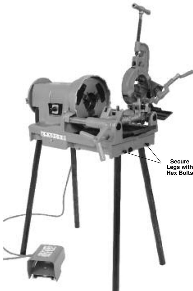
Figure 4 – Threading Machine Mounted On Pipe Legs
