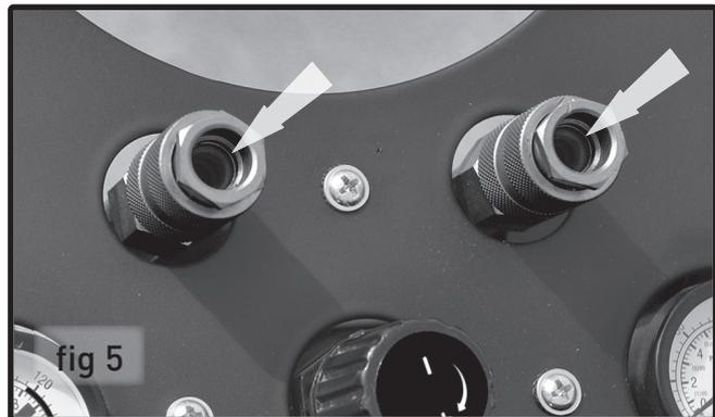
2. Verify that air hose is securely connected to air coupler by pulling on the air hose.
