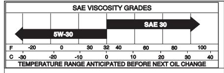
**CAUTION!** Although multi-viscosity oils (5W30, 10W30 etc.) improve starting in cold weather, these multi-viscosity oils will result in increased oil consumption when used above 32°F. Check your engine oil level more frequently to avoid possible engine damage from running low on oil.
