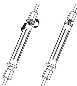
Make sure the drive control cable is not tensioned too tight. If the lawn mower starts to drive without the clutch lever is being operated, extend the wire.
