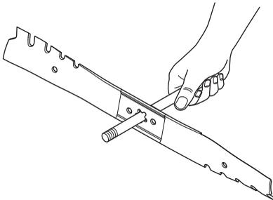
**IMPORTANT!** The blades should be balanced after sharpening. We do not recommend sharpening blade. Sharpening and balancing the blade should be conducted by an authorized service workshop.
