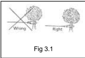
Locate a suitable anchor such as a strong tree trunk or boulder. Always use a sling as an anchor point. **⚠️ CAUTION** Do not attach the clevis hook back onto the cable as this could cause damage to the cable.
