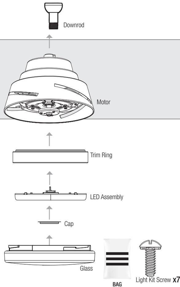
For installing the light kit
