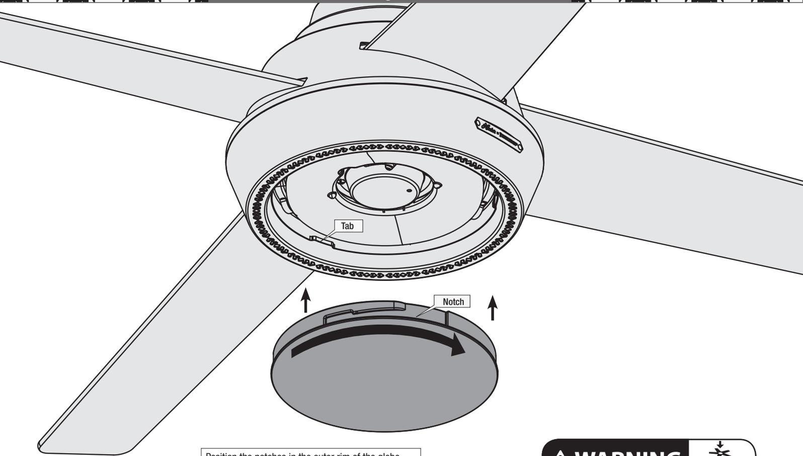
Position the notches in the outer rim of the globe so they line up with the three tabs on the inside rim of the housing. Carefully lift the globe up inside the housing as far as it will go, then rotate the globe clockwise until it is held tightly in place by the tabs.
