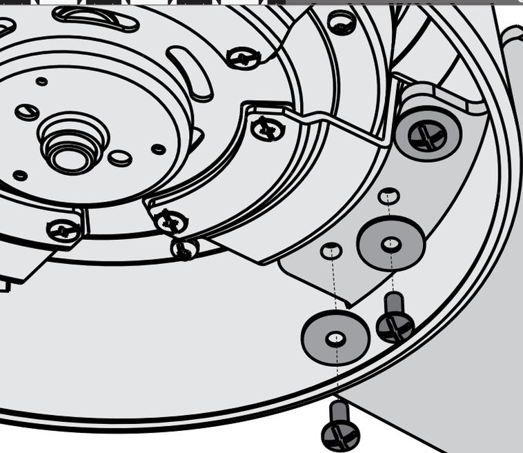
Attach each blade to a blade iron using three blade washers, found in the ■ hardware bag, and three blade assembly screws, found in the ▲ hardware bag.
