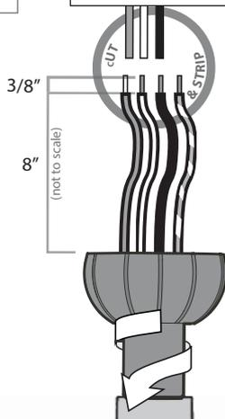
Pass all wires to one side of horizontal bar in downrod assembly. Hand tighten the downrod (at least 3-5 full turns) until it stops. Trim the wires coming from the fan so that 8-inches remain coming from the top of the downrod.
