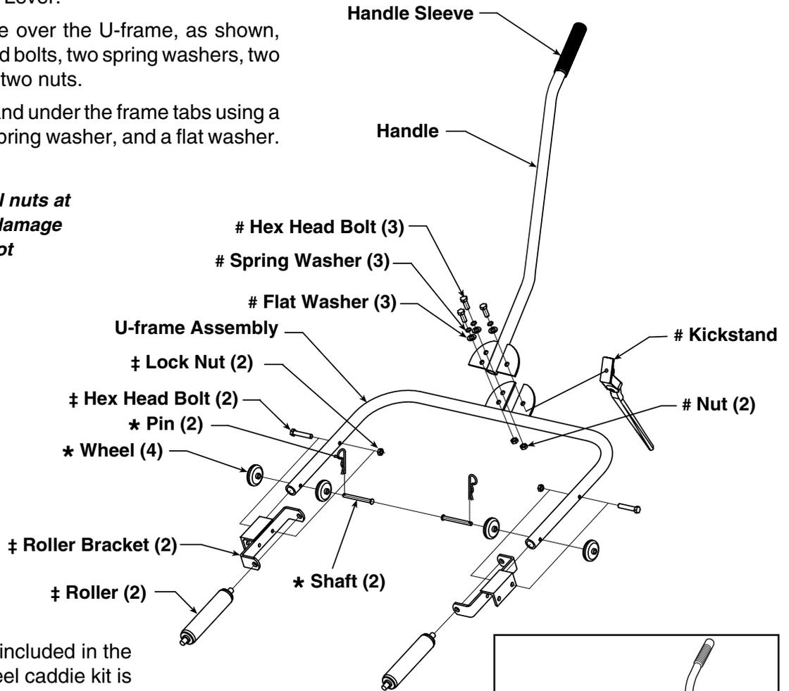
The number of parts included in the Easy Lift tire and wheel caddie kit is identified in parenthesis on the illustration. Parts not identified with a number are single units.
