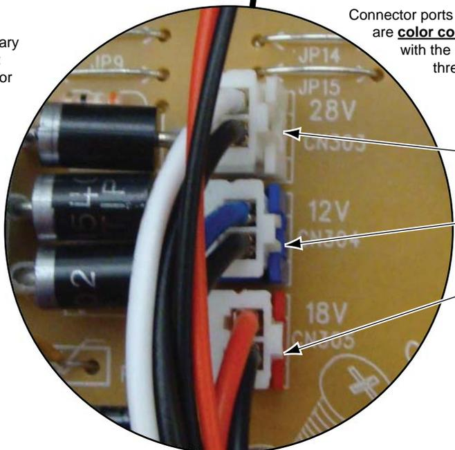
Connector ports on PCB Assembly are **color coded** to correspond with the colored wire of the three different voltage wire harnesses.
