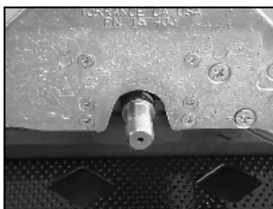
(N) Monthly, remove the Blade then clean and lubricate the Motor Shaft
