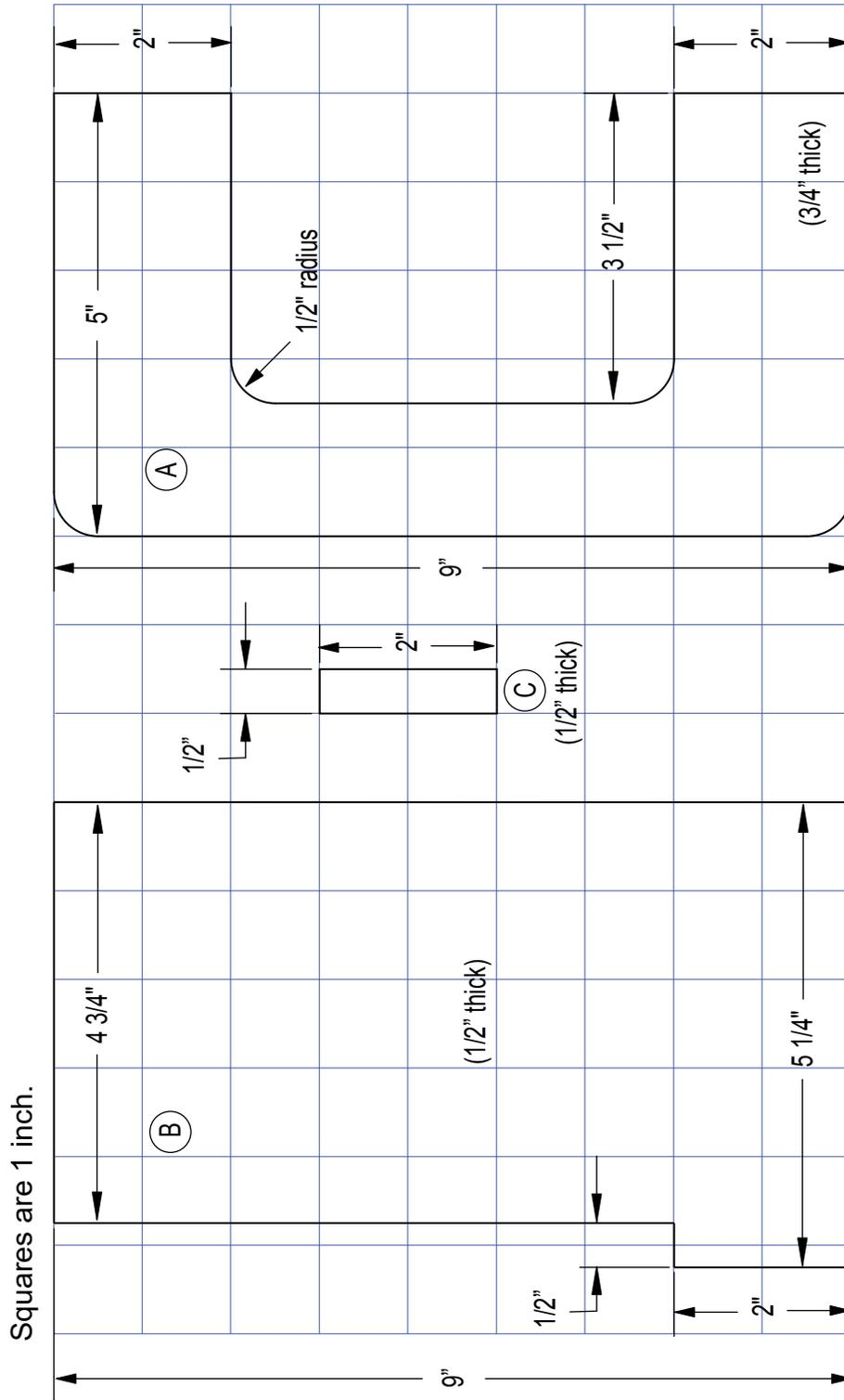
This diagram illustrates a typical push block. It includes the three pieces shown here labeled A, B, and C. Cut piece A out of 3/4 inch thick hardwood and cut pieces B and C out of 1/2 inch thick plywood. Attach piece A to the center of piece B using wood glue and counter-sunk wood screws. Attach piece C to piece B as shown in the drawing to the left using wood glue only. Do not use metal fasteners to attach piece C to piece B.
