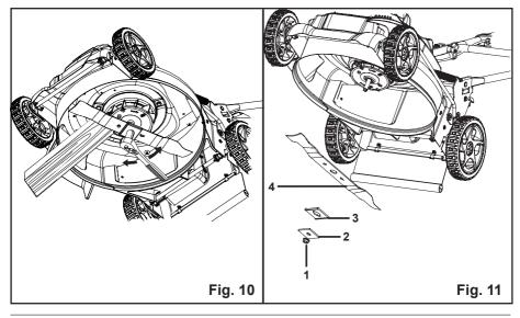
NOTE: Be sure to replace the parts in the exact order in which they were removed. When installing the cutting blade, verify that it is installed with the curved ends pointing toward the mower deck, and not toward the ground. Refer to the schematic drawing on page 26 of this Manual.
