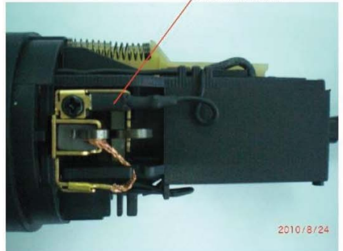
Black wire 'C' from field to left brush holder
