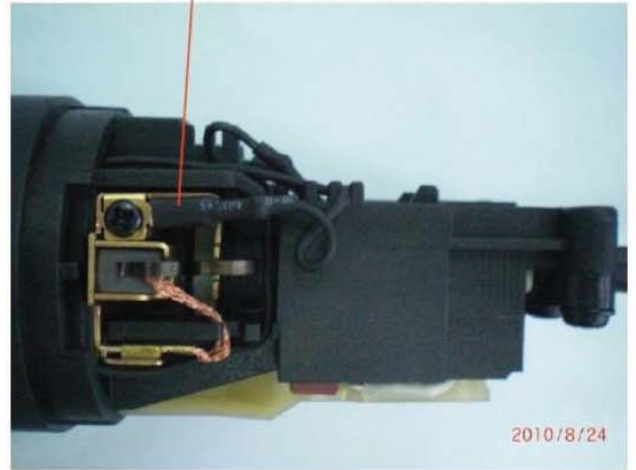
Black wire 'C' from field to left brush holder
