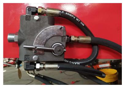
Adjust the rotating speed of the feed roller (from 0-600RPM).
