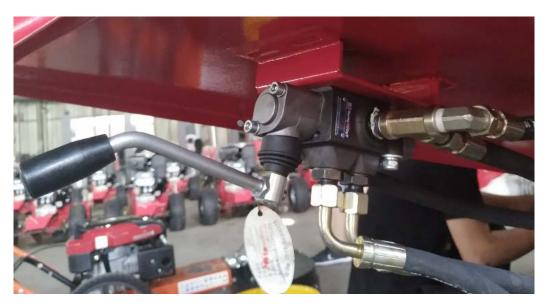
Control the FEED ROLLER: UP = reverse, CENTER = neutral, DOWN = forward feed
