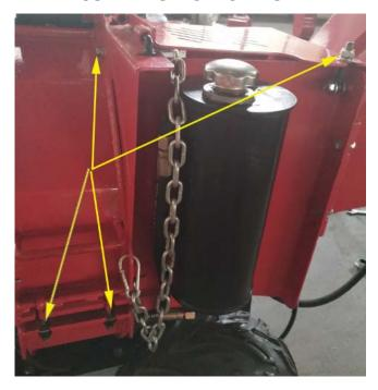
Loosen these 4 bolts, open the chamber to check the condition of blades and fans.
