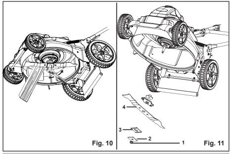
NOTE: Be sure to replace the parts in the exact order in which they were removed. When installing the cutting blade, verify that it is installed with the curved ends pointing toward the mower deck, and not toward the ground. Refer to the schematic drawing on page 27 of this manual.
