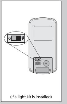
If a light kit is installed on your fan, choose the light bulb mode by moving the toggle switch. Move the switch towards the "D" for CFL bulbs and toward "ON" for standard bulbs. Replace the battery door.
