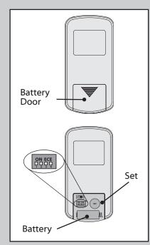
Remove battery door. Change the dip switch settings if the frequency matches a previously installed remote transmitter. Install A23 or MN21 alkaline battery in the proper polarity and replace the battery door. To pair the remote, hold down the Set button for 5 seconds. Pairing is complete when LED button flashes twice.
