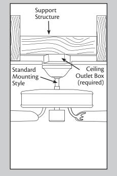
Use **Standard Mounting** or **Low-Profile Mounting** to hang the fan from a flat ceiling.
