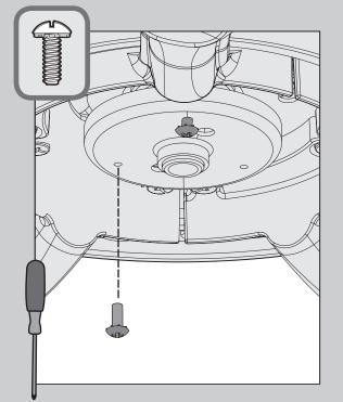
Screw two (2) housing assembly screws from the = hardware bag halfway into the mounting plate. It does not matter which two screw holes you choose.
