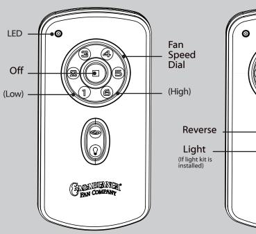
To select fan speed press one of the numbers on the Fan Speed Dial. To calibrate the fan speed, run the fan on "6" for 90 seconds after each AC power reset. The LED light flashes to indicate a signal has been sent to the fan.
