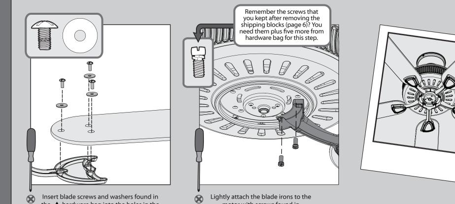
Insert blade screws and washers found in the ▲ hardware bag into the holes in the blades, then secure each blade to a blade iron. Lightly attach the blade irons to the motor with screws found in the ⊠ hardware bag, then securely tighten after both screws are attached.
