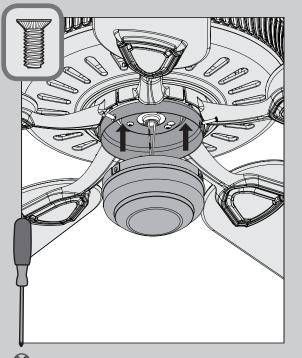
Lift the lower switch housing up until the holes line up with the screw holes in the upper switch housing. Install the three (3) switch housing screws, found in the = hardware bag.
