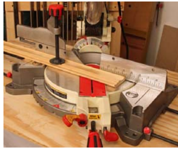
The spacious table (left) helps keep the wood stable during the cut. The handy scales (right) around the moveable miter table, at the bevel pivot and on the fence to make working faster and more accurate.
