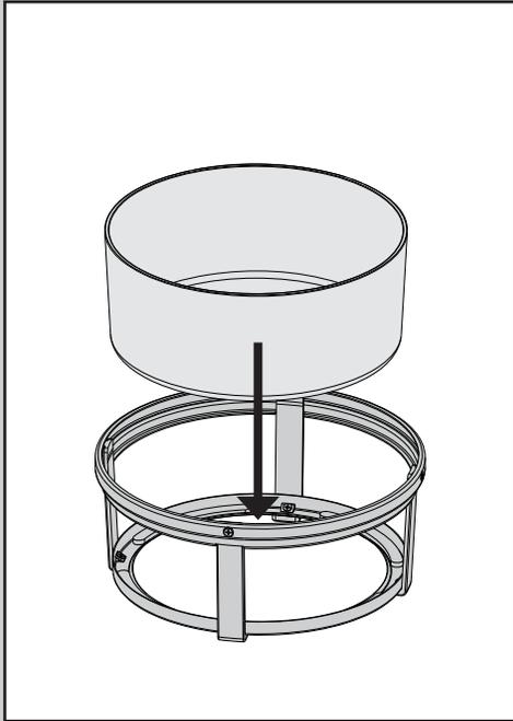
Carefully lower the globe into the globe retainer until it rests in place.
