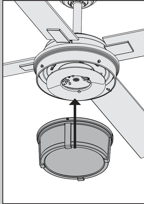
To install the cage and glass, first loosen the thumbscrews. Carefully raise the assembly to the light fixture and tighten all thumbscrews securely.
