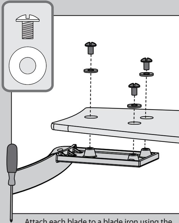
⊗ Attach each blade to a blade iron using the blade washers, found in the ■ hardware bag, and the blade assembly screws, found in the ▲ hardware bag.
