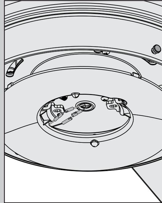
Connect the white wire from the fan to the white wire from the light kit. Then, connect the blue wire from the fan to the black wire from the light kit.
