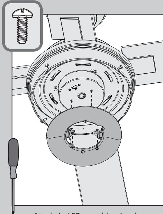
Attach the LED assembly using the LED assembly screws found in the hardware bag.
