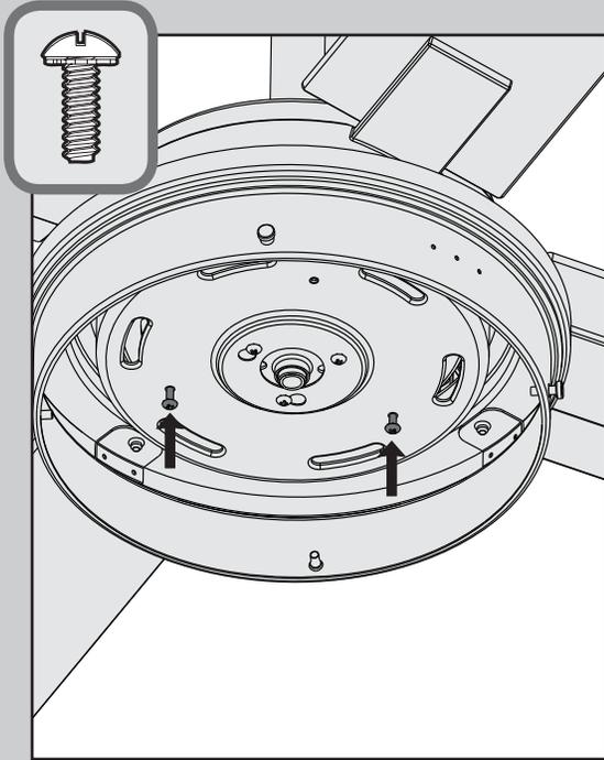
Partially install two of the switch housing screws found in the
