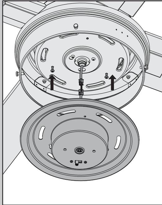
Connect the plugs from the upper and lower switch housings. Make sure to line up the colored markings on the connectors. Align the screw holes of the lower switch housing with the upper switch housing screws. Lift the lower switch housing. Twist the lower switch housing counterclockwise to lock into place.
