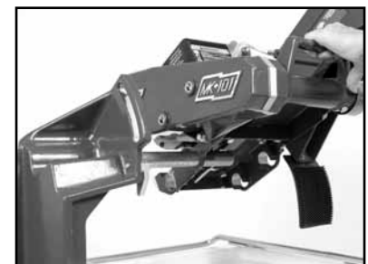
(I) Remove the Cutting Head (See Adjusting the Cutting Head).
