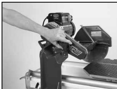
(A) Loosen Cutting Head Adjusting Knob.
