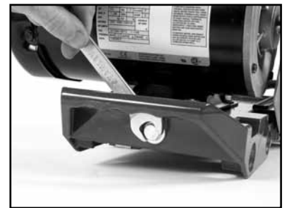
(I) Loosen the Motor Adjustment Strap
