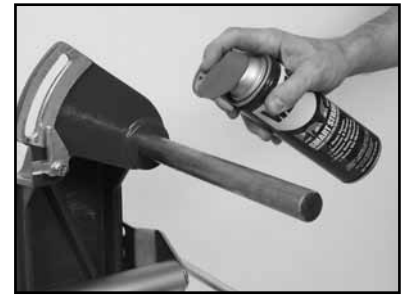
(L) Lubricate the Cutting Head Pivot Shaft.
