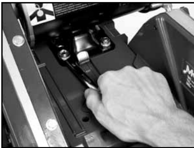
(P) Tighten the four motor mounting bolts
