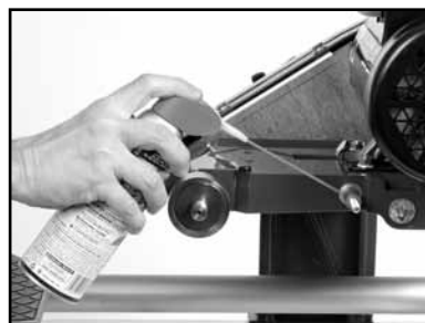
(H) Lubricate the Blade Guard Pivot Shaft.
