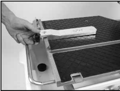
(A) Remove the Adjustable Cutting Guide.
