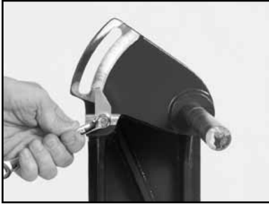
(A) Ensure Cutting Head Stop is in upward position.
