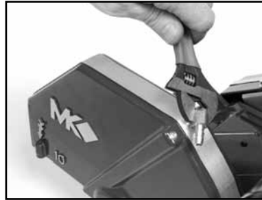
(E) Remove the Blade Guard Intake Fitting. Go to Step F.
