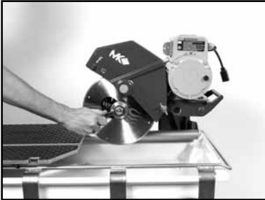
(A) Remove the Diamond Blade.
