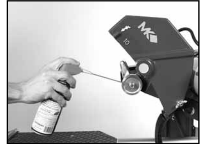
(C) Lubricate the Arbor Shaft.
