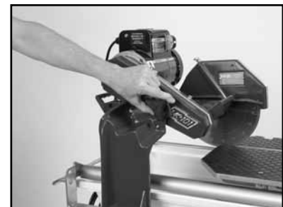
(C) Tighten the Adjusting Knob.
