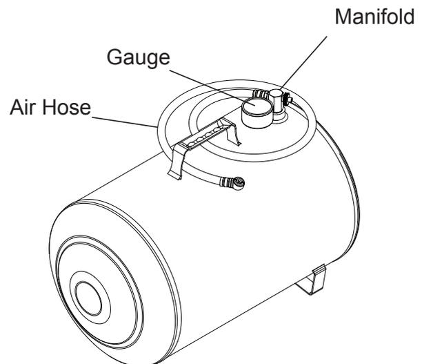
Figure 2 - Air Tank Replacement Parts
