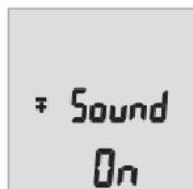
Press and hold the function button until you see the “Changing the Unit of Measure” display. Press the function button **4** again to see the image displayed to the left. Use button **3** and **6** to adjust the sound preference. **Sound OFF** will display when the sound has been turned off.
