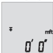
Press and hold the function button **4** until the image shown to the left is displayed. Use button **3** and button **6** to cycle through the units of measurement. Once the desired unit of measurement is displayed, press the measurement button **2** to return to measuring.
