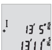
Press button **6** to add measured values or press button **3** to subtract measured values. “+” or “-” will appear in the middle of the display. Take another measurement. The current measured value will be shown at the bottom of the display, and the previous measured value will be shown above it.
