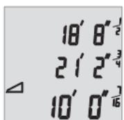
After the second measurement has been completed, the height will be automatically calculated and displayed. The end result will be shown at the bottom of the display, while the current measured value will be shown above it.
