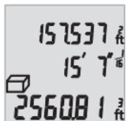
After the third measurement has been completed, the volume will be automatically calculated and displayed. The end result will be shown at the bottom of the display, while the current measured value will be shown above it.
