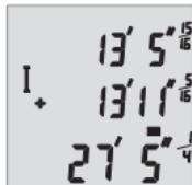
Press button **6** to add measured values or press button **3** to subtract measured values. The result will be shown at the bottom of the display after “=”, and the current measured value will be shown above it.
