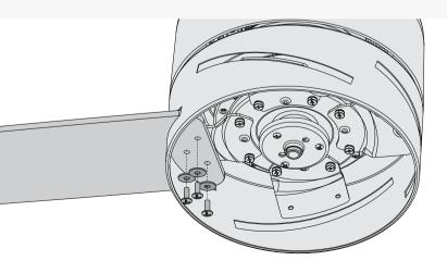
Put the blade washers found in the hardware bag onto the blade screws found in the hardware bag. Then install the blade screws to secure each blade to the fan.
