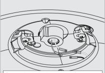
Connect the single-pin connectors from the LED assembly to the connectors from the fan. Connect the white wires together. Connect the blue and black wires together. Tuck the excess wiring above the LED assembly or feed back into the lower switch housing.
