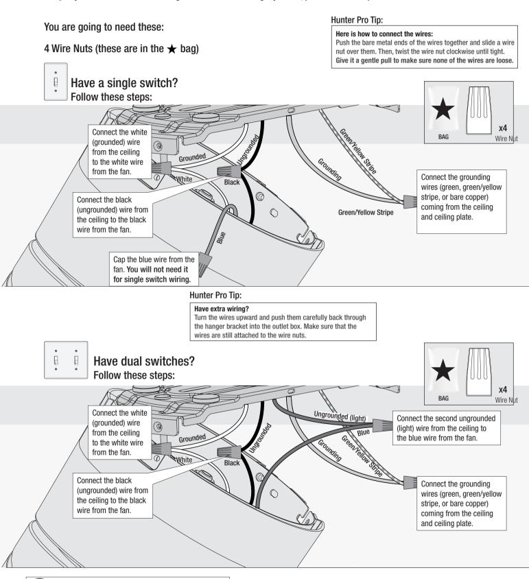
Ceiling Bracket Hanging Fan Wiring Installing Fan Body Blades Light Remote App
