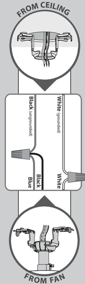
Using orange wire connectors from the ★ hardware bag, connect the black wire (ungrounded) from the ceiling to the black and the blue wires from the fan. Connect the white wire (grounded) from the ceiling to the white wire from the fan.
