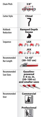
Long-lasting 70-series saw chain is designed for high performance, easy maintenance and loop consistency.
