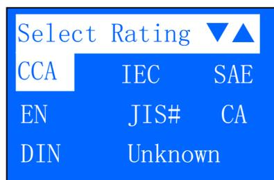
8. Select the rating system: CCA, DIN, EN, JIS#, IEC; according to the battery rating. If you cannot find its rating then select Unknown.
