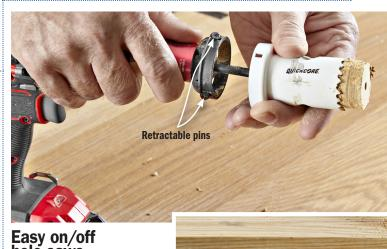
hole saws The unique quick-connect system of the Extreme Quickcore hole saws lets you change saws on the mandrel in a flash. Simply pull back on the mandrel sleeve, and the three pins retract to release the hole saw. To remove a cutaway plug from the hole saw, disconnect the saw from the mandrel and
