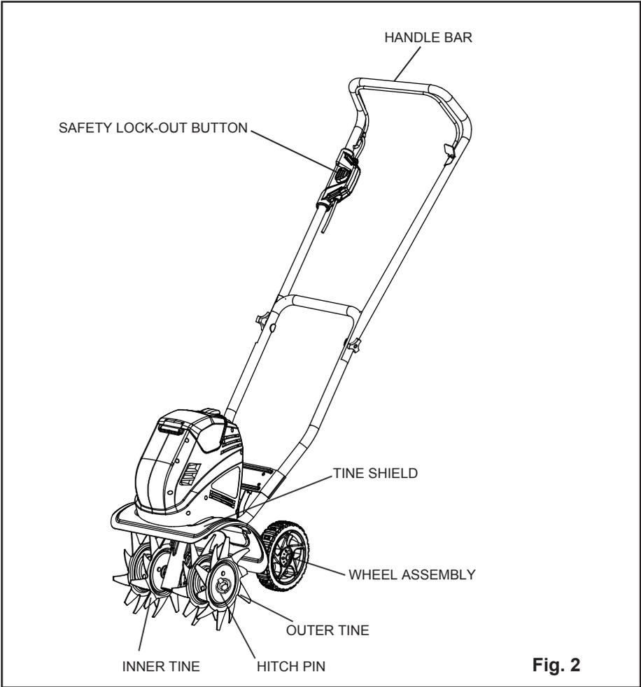
Read this operator's manual and safety rules before operating your cultivator. Compare the illustration in Fig.2.1 to your cultivator in order to familiarize yourself with the location of various controls and adjustments. Save this manual for future reference.
