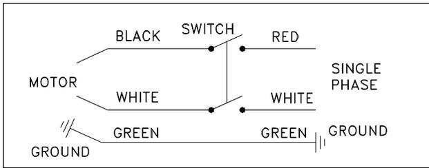
Figure 30: Schematic diagram for single phase motor.
