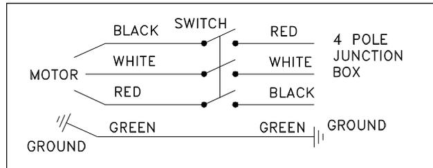
Figure 31: Schematic diagram for 3-phase motor.
