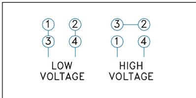
Figure 32: Motor connection diagram for 1-phase motor.
