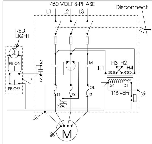
Figure 27 and 28, below: Wiring diagrams for 230 and 460 VAC with push button switch.
