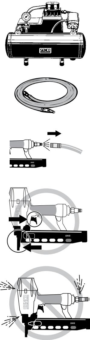
**DANGER** (1) Read and understand tool labels and instructions. (2) Wear eye protection. (3) Others in work area MUST wear safety glasses with side shields. (4) When driving fasteners to avoid accidental firing. (4) See manual (5) NEVER point tool at yourself or others in work area. (6) NEVER use oxygen or other gases. (7) MAX AIR PRESS. 120 PSI (8.3 BAR)
