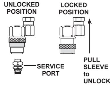
To attach to the system, make sure that the coupler is in its unlocked position. Press the coupler against the service port until it snaps (locked position).
