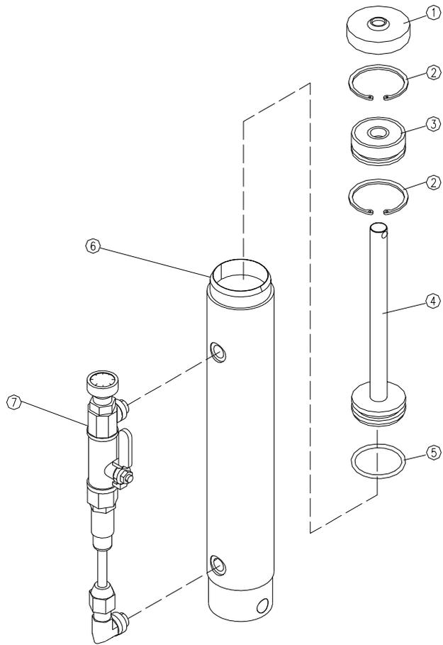
Figure 18: Hydraulic control cylinder exploded view
