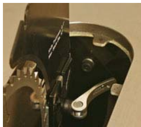
The quick-release mount for the riving knife follows the blade so critical alignments remain constant.
