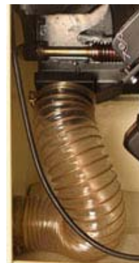
A 4”-diameter flex hose connects the internal shroud to the 4”-diameter external port.
