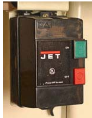
JET motors (left) are rated for continuous duty cycle, no “peak” or “max developed”. This rating insures you get all of the power listed! The magnetic switch, (right) while costly does a lot to protect the motor and you when the power becomes unstable.
