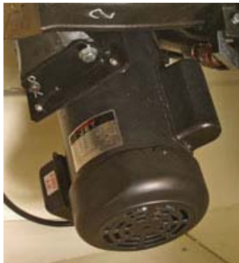
JET motors (left) are rated for continuous duty cycle, no “peak” or “max developed”. This rating insures you get all of the power listed! The magnetic switch, (right) while costly does a lot to protect the motor and you when the power becomes unstable.
