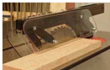
The independent “leaves” on the blade guard allow one to ride up on the wood and the other to remain flat on the table during narrow cuts to contain more debris and enhance dust collection.
