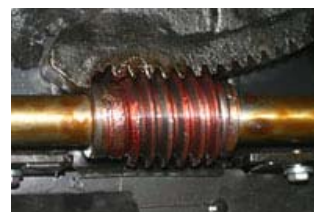
Smooth-operating, precisely machined worm gears handle blade height and bevel adjustments.
