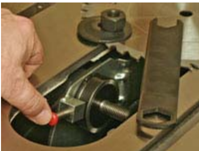
The pushbutton arbor lock and offset wrench make changing blades easy and safer.
