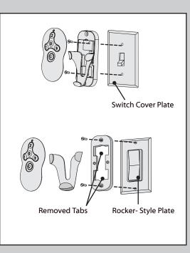
To install the transmitter cradle, remove the two screws holding the switch cover plate. Do not remove the cover plate. Orient the cradle by lining up the two mounting holes with those on the cover plate. Insert and tighten the screws. Do not over tighten. **Note:** For rocker-style cover plates, break off the tabs by pushing outward.
