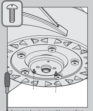
Screw two housing assembly screws from
