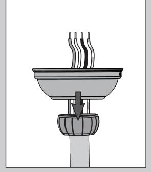
Put the wires and downrod through the canopy. Let the canopy sit loosely on top of the fan.
