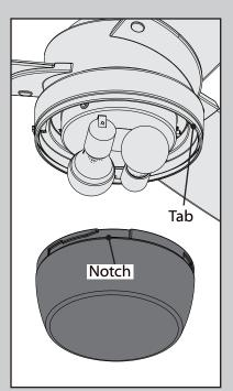
Lift the globe and align the notches in the globe with the tabs in the light kit. Attach the glass bowl to the light kit by twisting it clockwise until it snaps into place.
