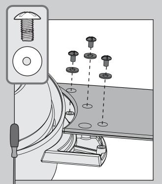
Attach each blade to a blade iron using three blade washers, found in the hardware bag, and three blade assembly screws, found in the hardware bag.
