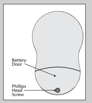
To access the battery compartment, remove the small Phillips head screw that secures the battery door to the transmitter assembly. The battery should be installed with the positive (+) side up. Replace with a CR2032 battery when necessary.
