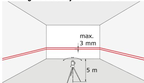
Place the lock switch in the "Unlocked" position (see [Levelling lock](#)). Position the instrument approx. 5 m away from the wall. Direct the instrument at the wall and switch on. Activate the laser line and mark the intersection point of laser crosshairs on the wall. Swivel the instrument to the right and then to the left. Observe the vertical deviation of the horizontal line from the marking. If the difference does not exceed 3 mm, then the instrument is within tolerance.
