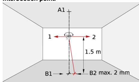
Place the lock switch in the "Unlocked" position (see [Levelling lock](#)). Set up the laser on its tripod or wall mount bracket near point A1 at a minimum distance of 1.5 m from point B1. The horizontal laser is aligned in direction 1. Mark the laser points A1 and B1 with a pin.
