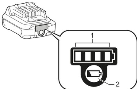
Press the check button (2) on the battery cartridge to indicate the remaining battery capacity. The indicator lamps (1) light up for a few seconds and show the remaining capacity:
