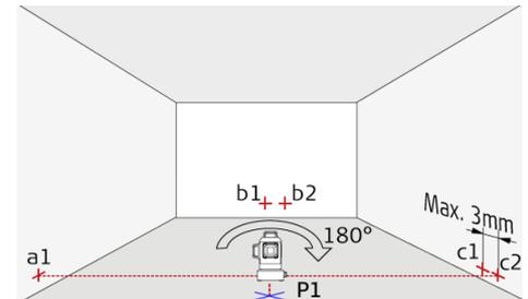
Afterwards, turn the instrument exactly 180° around the plumb intersection point P1 and position the plumb intersection point to the existing reference point a1. Make sure that the lower intersection plumb point is still exactly on the reference P1. Then mark the left-hand beam to the right wall and mark it with c2. Finally measure the difference between the former reference point c1 and the new point c2. The deviation may be max. 3mm between these two points.
