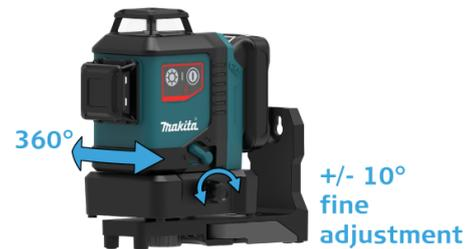
Turn the instrument 360° to adjust the vertical line. Use the fine adjustment knob and turn the instrument around the vertical intersection / plumb point within  $\pm 10^\circ$ .
