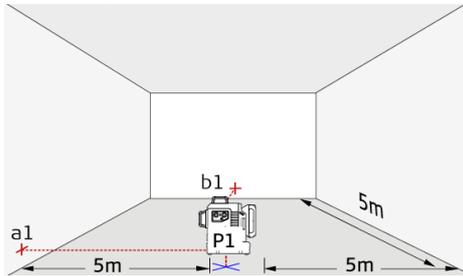
Place lock switch in "Unlocked" position (see [Levelling lock](#)). Mark a reference point (P1) approx. 5m from the walls and position the lower plumb intersection point exactly on it. Align the cross hair to the left wall and mark the intersection point (a1) approx. on the same height like P1 to the wall. Shortly after mark the right-hand perpendicular beam (b1) on the front wall.
