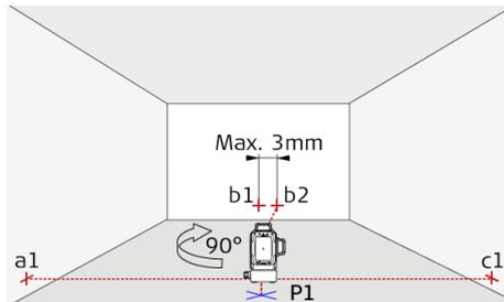
Then rotate the instrument exactly 90° clockwise around the plumb intersection point P1 and position the left-hand perpendicular intersection beam to the existing reference point a1. Make sure that the lower plumb intersection point is still exactly on the reference P1. Check afterwards the new reference point b2 with the old reference b1 on the front wall. The deviation between the two points may be max. 3mm. Mark the new position of the right-hand perpendicular beam to the right wall with c1.
