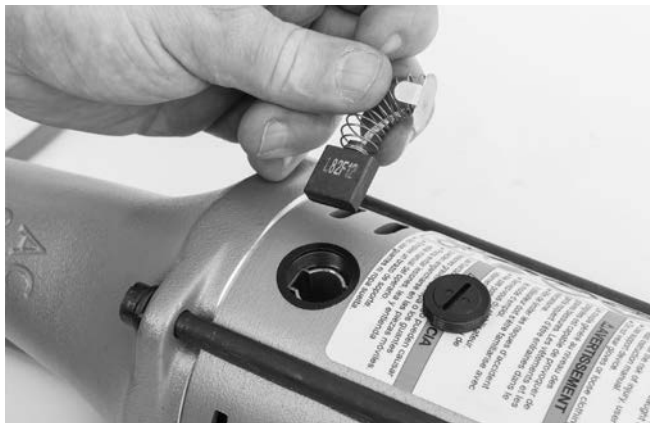
Figure 13 – Installation des balais
