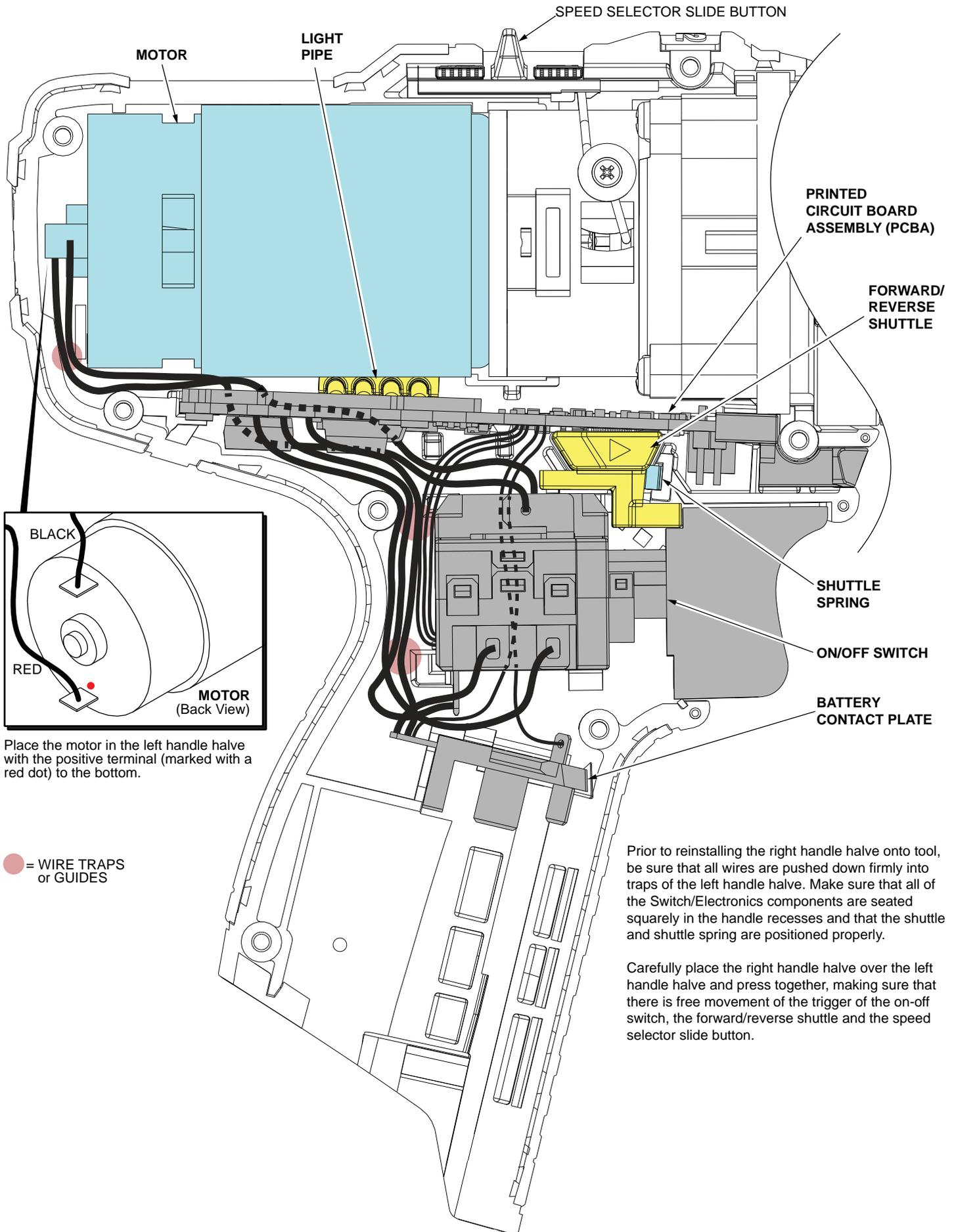
Place the motor in the left handle halve with the positive terminal (marked with a red dot) to the bottom.
