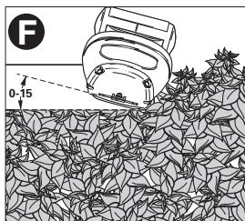
**CAUTION:** Do not use trimmer for cutting stems greater than 5/8 in. (16mm). Use the trimmer only for cutting normal shrubbery found around houses and buildings.
