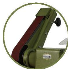
Belt Grinder Side Adjustable in Height
