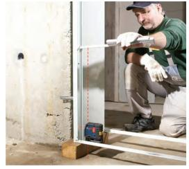
**PLUMB AND LEVEL POINT PROJECTION**Accurately transfers and aligns level, plumb, 90-degree and grade points
