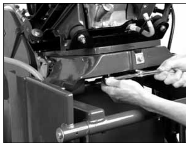
(K) Tighten Engine Mounting Plate.
