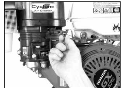
(C) Move the Throttle Lever to 1/3 open.
