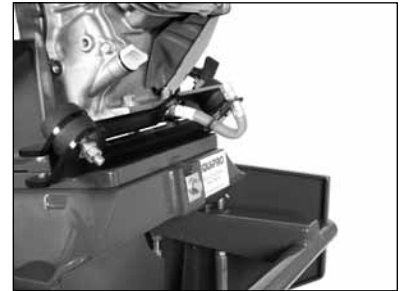
(C) Fill Oil Reservoir. (See Engine Manual)
