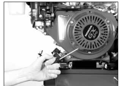
(F) Pull Starter Cord slowly, until slack is removed and resistance is felt.
