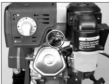
(B) Replace Spark Plug. (See Engine Manual)
