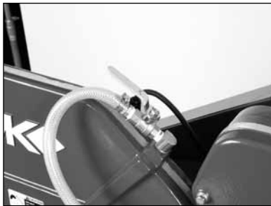
(A) Check Cooling Flow Control Valve is open.
