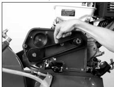
(B) Check and adjust the Blade Shaft Belt and Jack Shaft belt tension following first 48 hours of operation. (See Belt Inspection)
