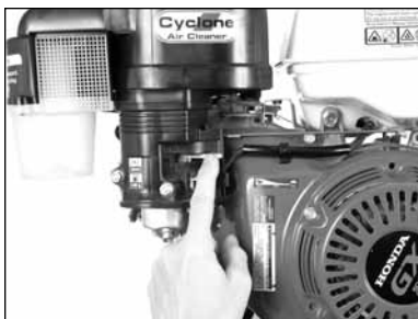
(H) Place Choke Lever in the OPEN position when engine is warm.
