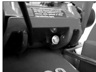
(I) Tighten the Engine Adjustment Strap Bolt to remove slack.
