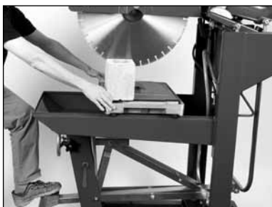
(E) Repeat Steps C and D until cut complete. Turn the saw off when work is complete.
