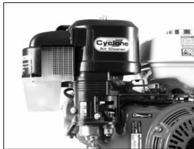
(H) Check Air Filter for cleanliness. (See Maintenance section if dirty)
