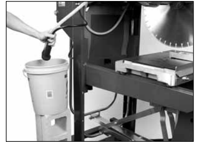
(C) Place the Water Pump Assembly into an external water source container. Fill the external water source container and place a catch basin below the Drain Hole.
