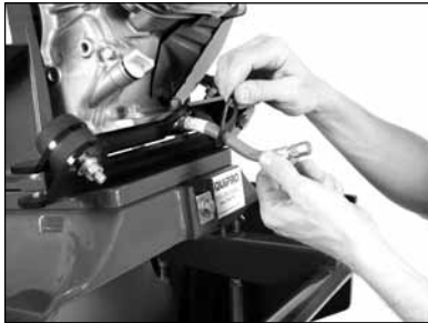
(A) Raise Cutting Head. Straighten oil drain hose.
