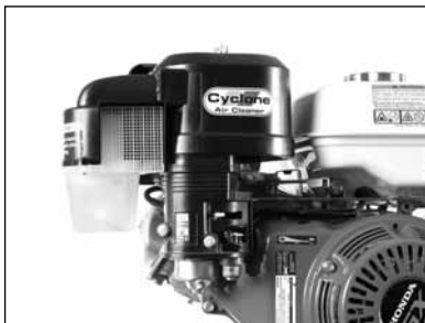
(A) The Air Filter needs to be cleaned and/or replaced occa- sionally. (See Engine Manual)
