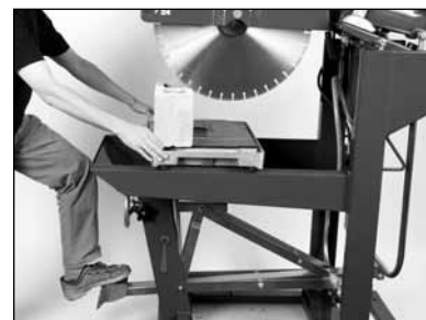
(C) Step Cut "Push" Stroke. Lower Cutting Head 1/4" - 1/2" during Push Stroke.
