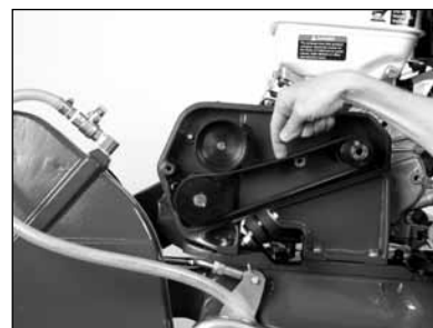
(C) Check Belt for proper tension. If tension is correct, go to step K check tension 1/2-way between pulleys (proper tension 1/8" deflection).
