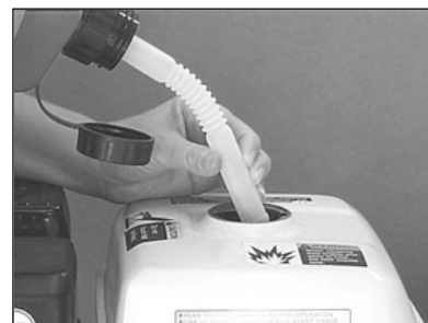
(C) Fill Fuel Tank until level is below throat.
