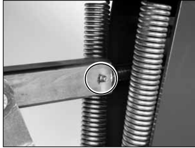
(H) Depth Control Screw Housing lubrication point.
