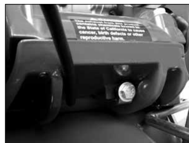
(C) Verify engine Adjustment Straps are tight.
