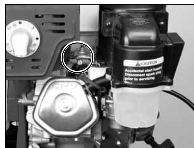
(C) Clean and readjust engine Spark Plug (See Engine Manual)
