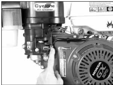
(A) Place Fuel Valve in the ON position.
