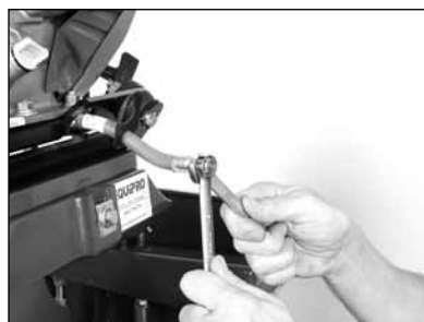
(A) Change engine oil. (See Engine Manual)
