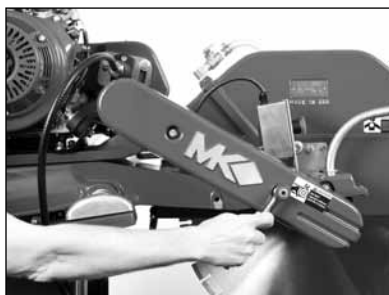
(A) Remove the Belt Guard Retaining Bolts.
