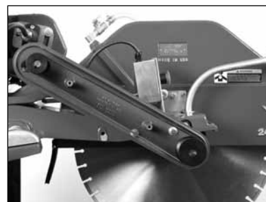
(C) Inspect belts. (See Belt Inspection, Adjustment and Replacement)
