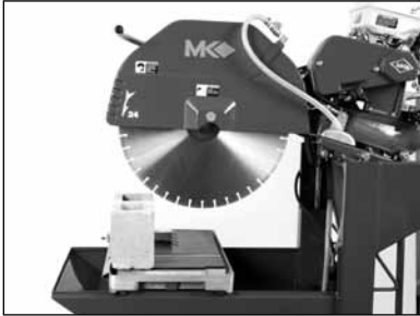
(A) Adjust the height of the Cutting Head as necessary, start engine.
