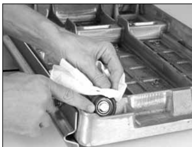
(E) Clean the Movable Cutting Table Roller Wheels.
