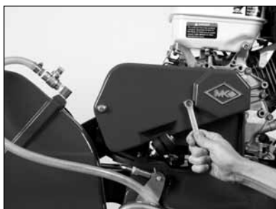
(A) Remove the Belt Guard Retaining Bolts.
