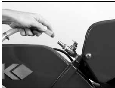
(B) Remove Transfer Tube from Blade Guard.
