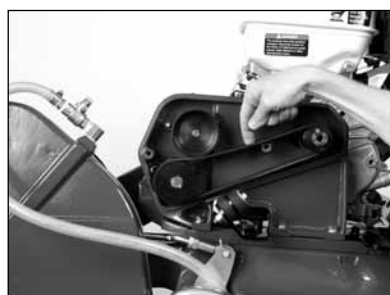
(J) Check belt tension (proper tension 1/8" deflection of the belt). Continue adjusting belt until tension is correct then tighten the Engine Plate Mounting Bolts.
