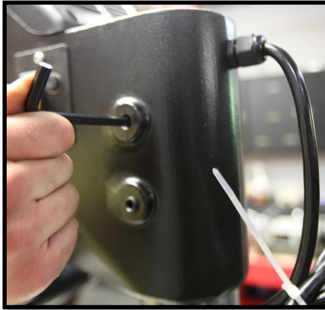
Figure 5 - Mounting the headstock
