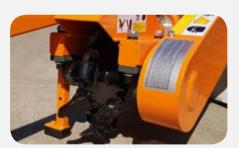
9 Carbide Cutting Head - Direct Drive
