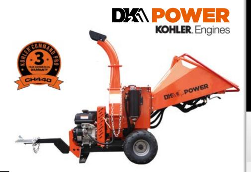
5" Electric Start chipper self contained auto feed system with hydraulic roller speeds up to 600 rpm.
