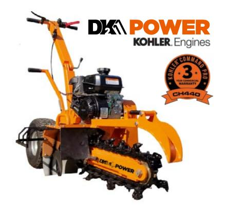
Direct Chain Drive Trencher. High pressure sintered carbide teeth. 5 depth positions, dual locking wheels for digging in reverse. 3/8 plow plates with quick change teeth. Adjustable handle, Keyed safety lock out, 6 inch direct drive auger. Heavy gauge steel construction.
