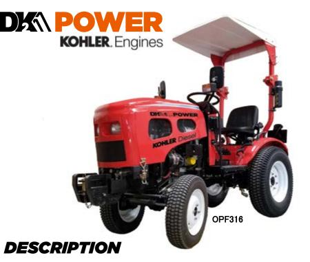
This unit sports plenty of torque at 3900 force (N). The quick response 540 rpm to 1000 rpm PTO drives 4 and 5 foot CAT1 implements with ease. Turf tires make this a versatile tractor for lawn, garden, and field work.
