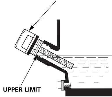
3. Reinstall the oil filler cap.
