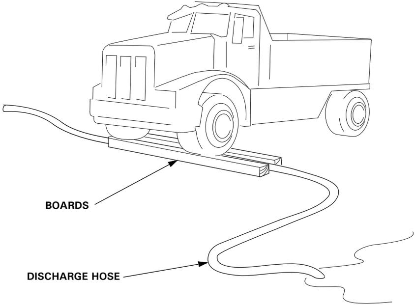
Driving over a discharge hose while the pump is running, or even possibly when the pump is stopped, may cause pump case failure.
