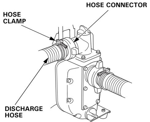
Tighten the hose clamp securely to prevent the discharge hose from disconnecting under high pressure.
